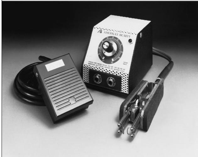
The ease and simplicity of operation of the Thermal Wire Stripper make it ideal for most strain gage leadwire stripping. The variable heat control allows stripping of all thermoplastic insulations, including Teflon®, in sizes No. 18 to No. 36 AWG (1 to 0.1 mm diameter). The foot switch and tweezers hand-piece give excellent operator control over the stripping operation. Includes power unit and foot switch, both with 3-wire NEMA plugs, and tweezers handpiece.
