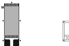
Longer grid for strain averaging or where higher power dissipation is required.
