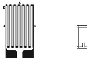
Large grid and high resistance permit higher-than-normal excitation voltage.
